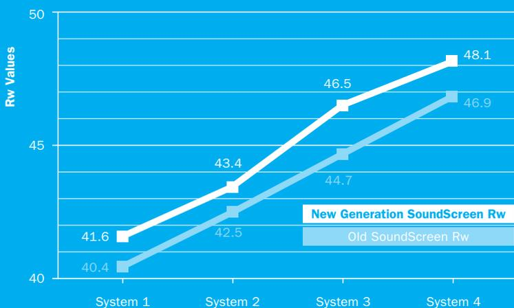
System 1 – 90mm Timber stud with 70mm SoundScreen and 1 x 10mm Standard CSR Gyprock Plasterboard both sides
