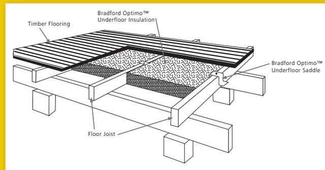
Bradford Optimo™ segments are most easily installed from above before the floor is installed.
