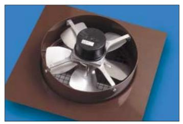
**ecoFAN** is a quality manufactured Australian product consisting of a heavy duty electronic D.C. brushless motor, 23 cm diameter fan and rustproof aluminium frame.
